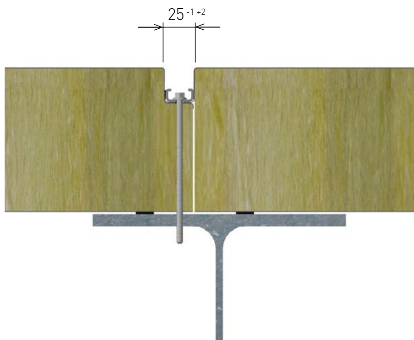
Fig. 3.6: Permissible tolerances of the vertical joint
