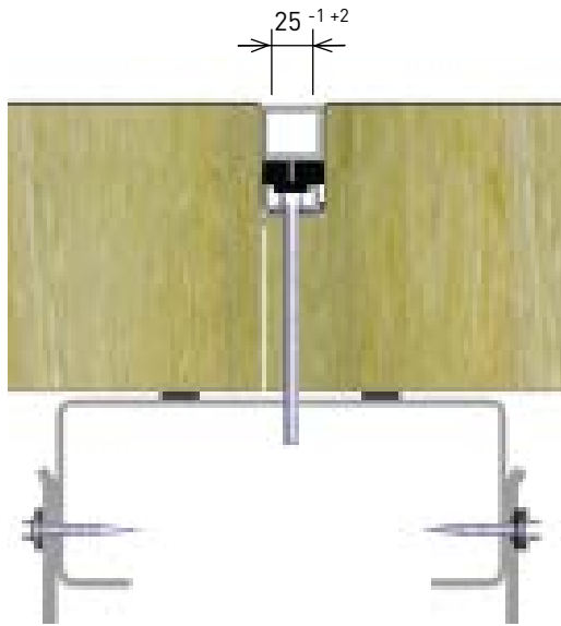
Fig. 1.6: TRANSVERSAL and LONGITUDINAL joint for both horizontal installation methods
